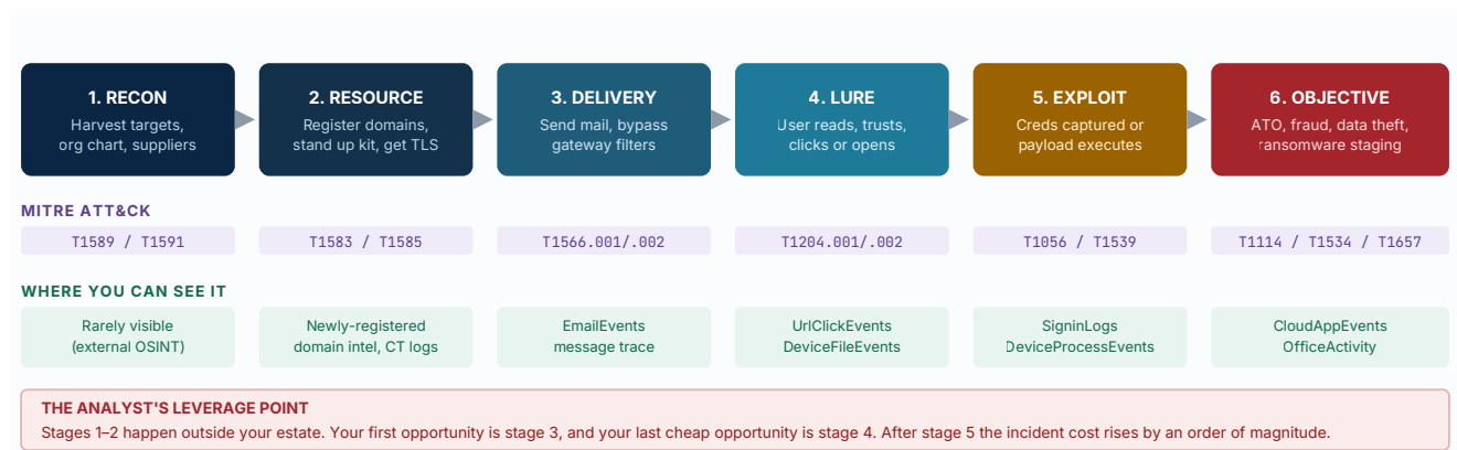
Figure 3.1— The phishing attack chain , mapped to ATT&CK techniques and to the telemetry where each stage becomes observable. Investigation is the art of pulling the timeline as far left as possible.
